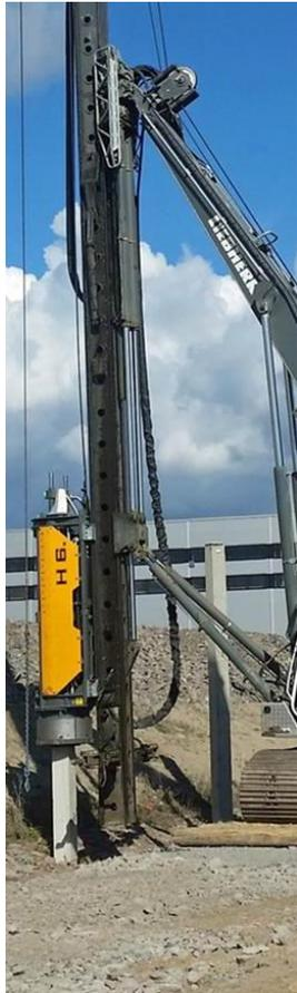
**Evaluate** use of hydraulic vs diesel hammer
