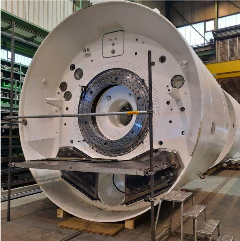
Tunnel Boring Machine Front Shield
