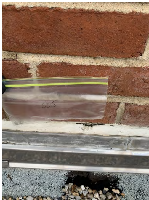
Photo 8 - Sample 005 beige caulking between brick and flashing 5% Chrysotile ACM
