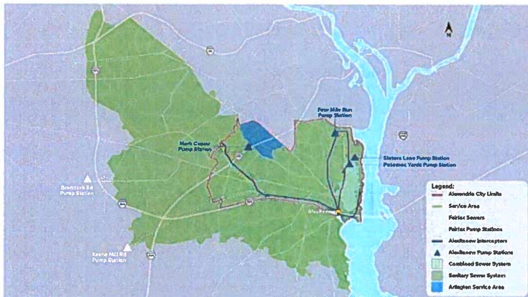
Under dry weather conditions flows collected in the CSS are conveyed to AlexRenew's WRRF. During periods of rainfall, the capacity of the CSS is exceeded and combined sewer flows are discharged directly to Hunting Creek, Hooffs Run, and the Potomac River through four permitted outfalls.
