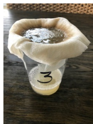
Solids gathering on top of paper towel while water filters through to cup 3.
