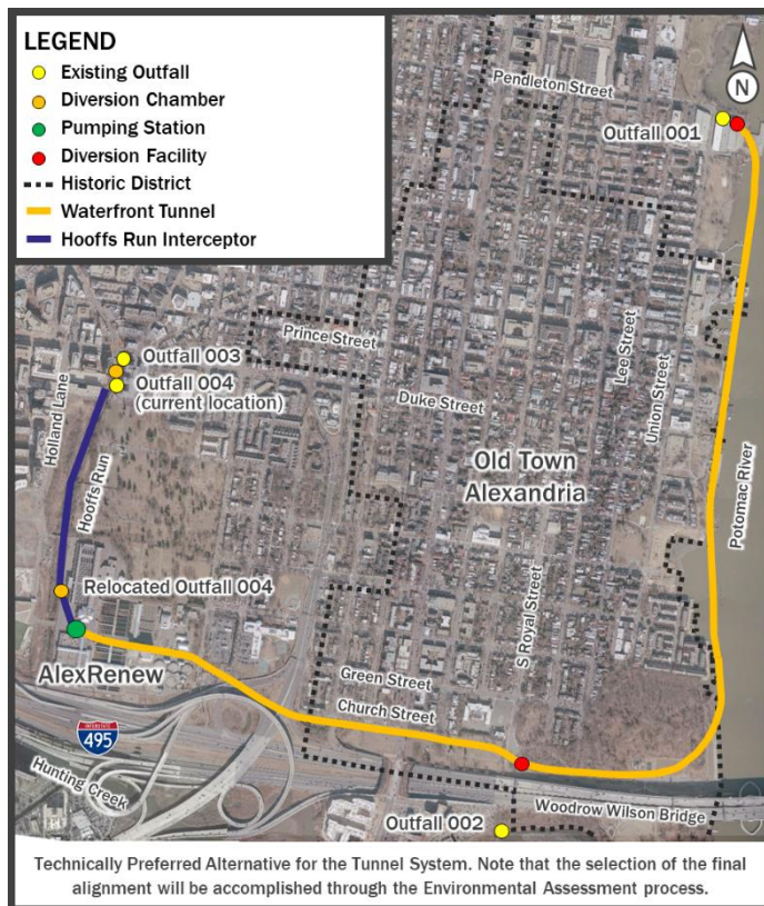
Figure 2.2. Tunnel System Project Major Components
